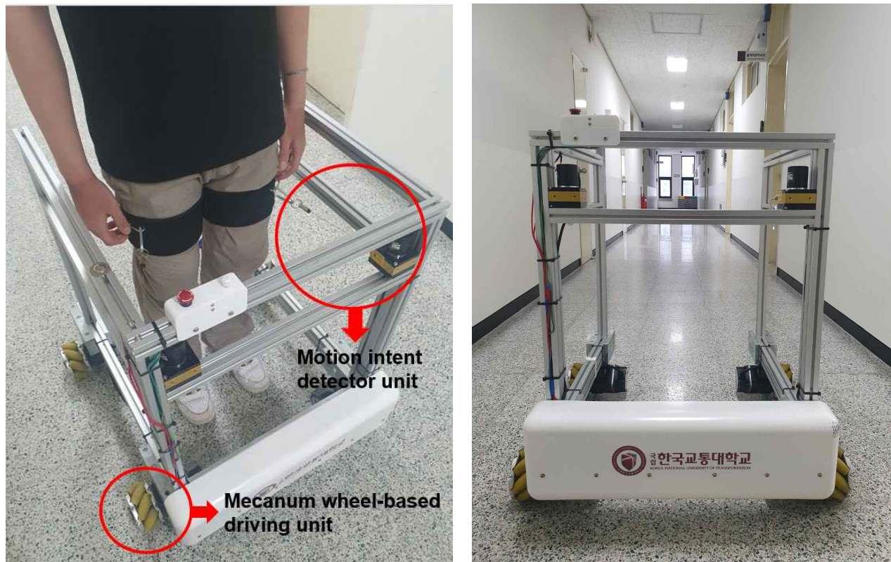
Figure 1. Setting for the motion tracking gait assistive walker
