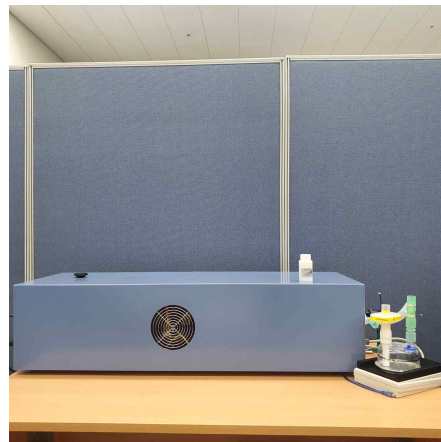
Figure 6. ATS 24/26 waveform test of “The Spirokit”
