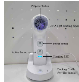
Figure 5. Main components of “The Spirokit”
