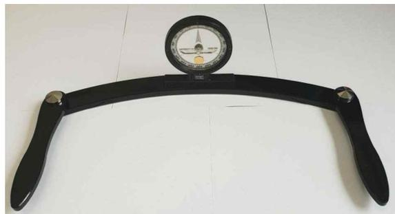
Figure 1. Baseline AcuAngle Inclinometer
